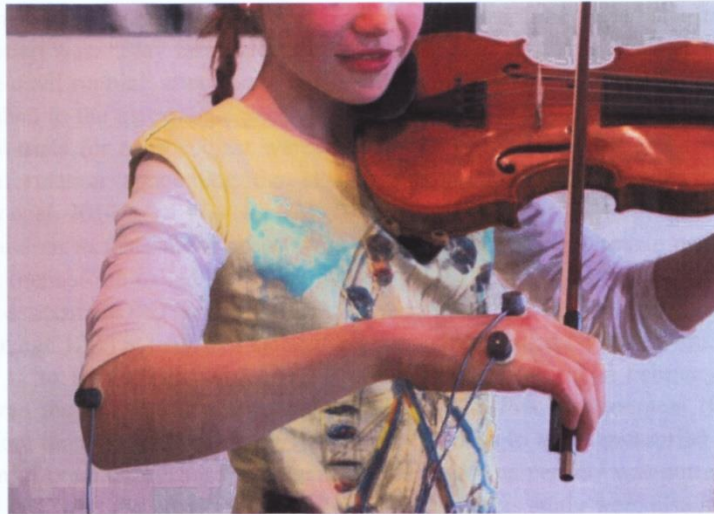
Figure 2. Violin student in the three-dimensional measurement of her bowing movement using the ultrasonic system Zebri CMS 20 (Zebri Medical, Isny, Germany).
