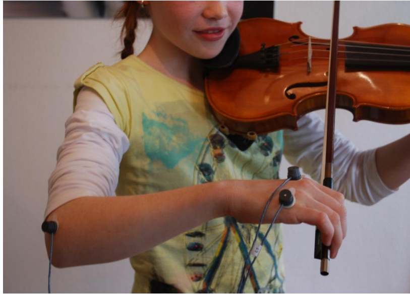
Figure 2. Violin student in the three-dimensional measurement of her bowing movement using the ultrasonic system Zebbris CMS 20 (Zebbris Medical, Isny, Germany).
